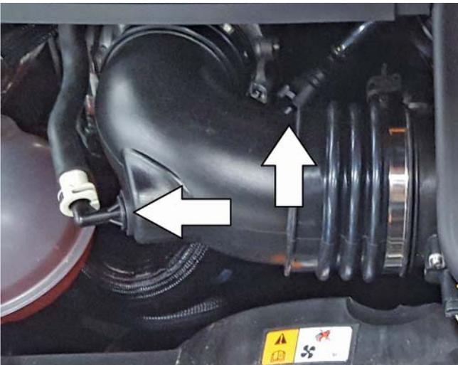
12. Remove the MAF sensor from the factory air box by removing the two (2) T-15 torx screws.
