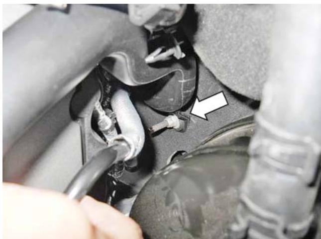
14. Using a trim tool, pry up on the push pin retaining the induction resonance tube and remove the tube from the vehicle.
