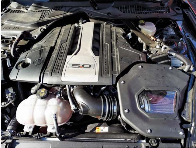
16. Re-install the engine cover and strut tower brace. Torque to engine cover to 10 Nm and the strut brace to 55 Nm.
