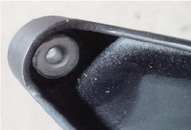
3. Install the second grommet onto the air box (P/N: 131550-9A612).
