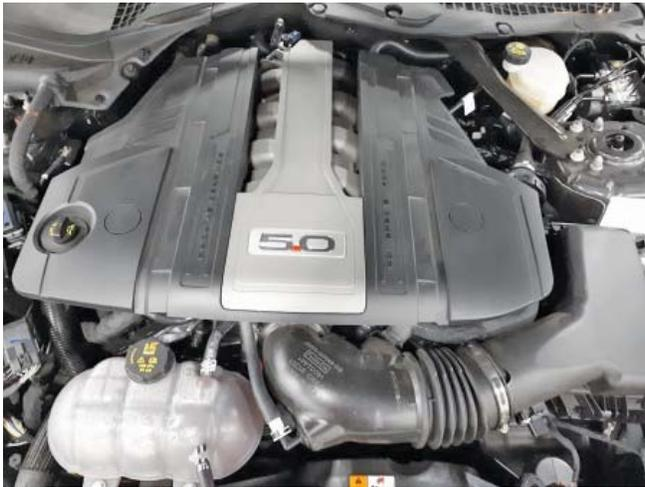
4. Remove the plastic caps exposing the fasteners holding the cover down. Unbolt the cover and pull up to remove it from the grommets.
