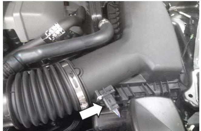
6. Loosen the clamp at the air box from the intake tube.
