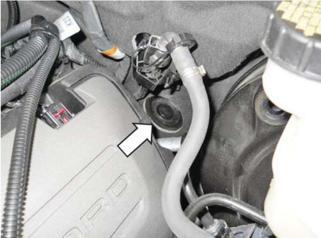
2. Install the grommet and sleeve that was removed from the stock air box into the ROUSH air box (P/N: 131550-9A612). **TIP:** Install the rubber grommet first, then install the steel bushing.
