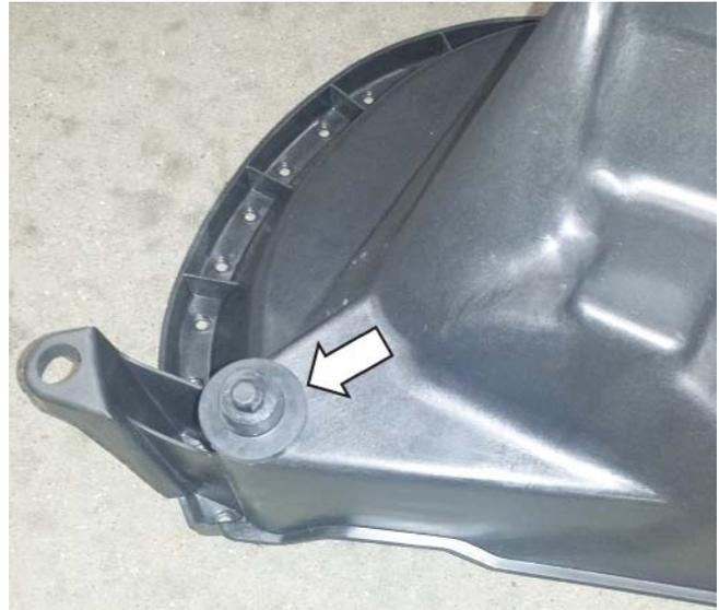
4. Install the rubber isolator into the bottom of the air box (P/N: 131550-9A612).
