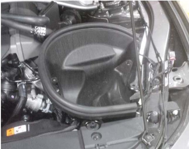
7. Using a 10 mm socket and the bolt removed from the stock air box, attach the air box to the vehicle. Torque to 8 Nm.
