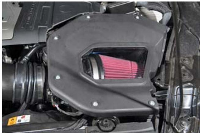
15. Use template on the back page to trim the engine cover. (Use the measurement on the diameter to verify template sizing.)
