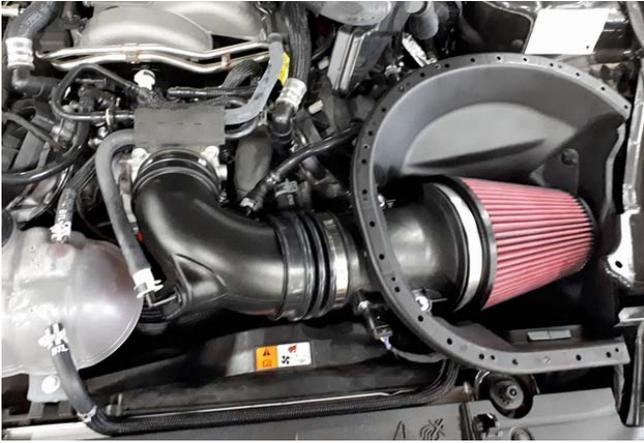
11. Reconnect the two (2) hoses with quick connect fittings to the mating push-on barbs.
