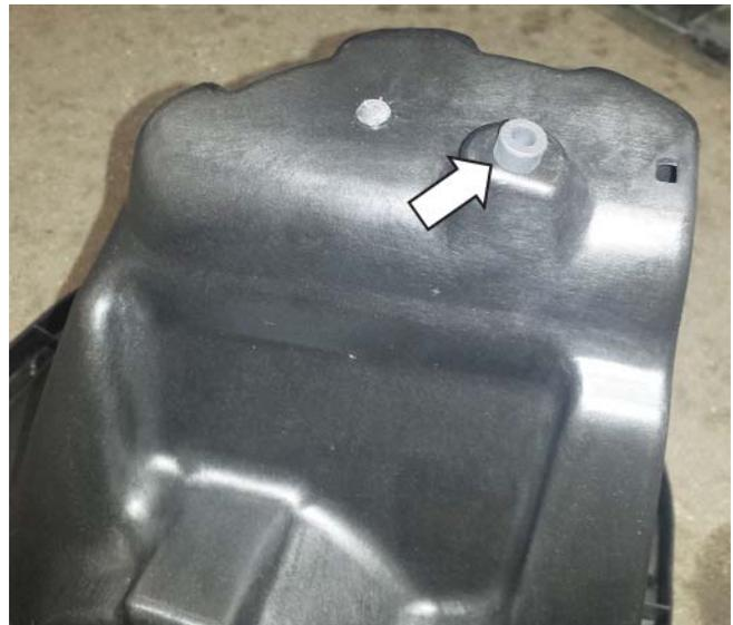
5. Insert the dirty air inlet (P/N: 1315-9F763-A) into the air box (P/N: 131550-9A612).
