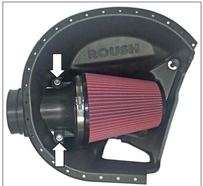
10. Install the clean air tube assembly (P/N: 131550-9R504) onto the throttle body first and then the filter tube. Tighten the clamps to 3 Nm.
