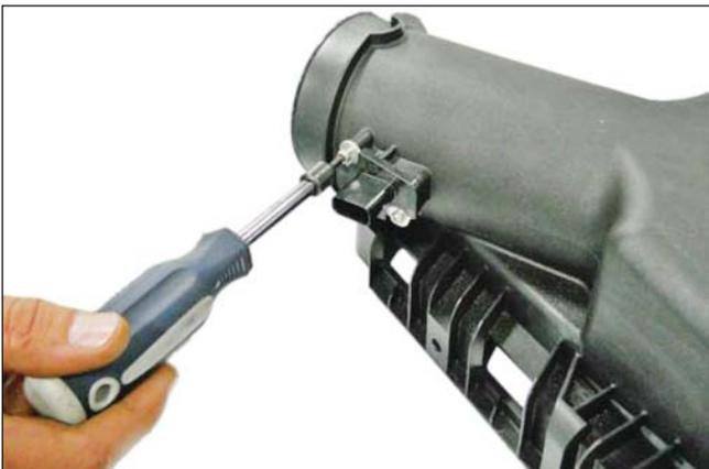
13. Re-install the MAF sensor into the ROUSH filter tube (P/N: 131550-12B579). Reattach the connector. Torque screws to 2 Nm.
