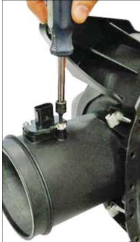
14. Install the lid onto the airbox assembly (P/N: 1318-9643HC-AA) Use six (6) self tapping screws (P/N: W506976-S437) to secure the lid.
