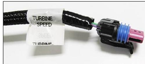
Figure 31 - Turbine Speed Sensor
