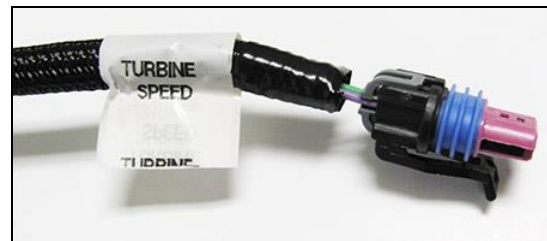
Turbine Speed Sensor
