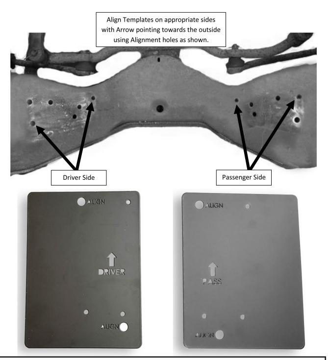
Place Templates on Appropriate sides with the Arrow pointing upwards
